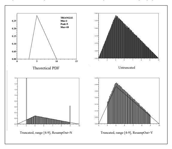
Figure 3.12. The Triangle Distribution in APEX
