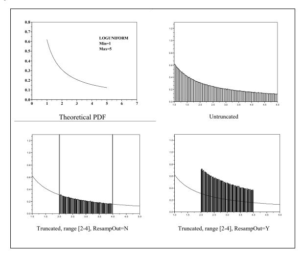
Figure 3.9. The Loguniform Distribution in APEX
