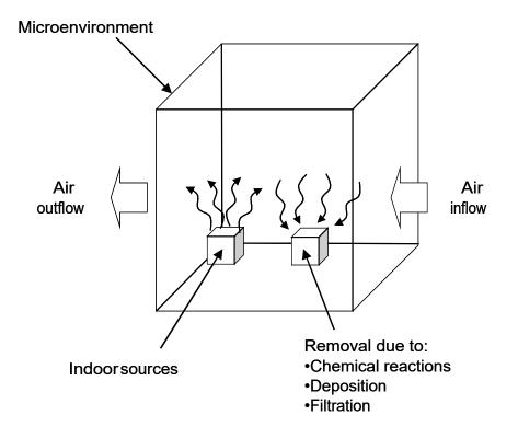
Figure 8.1. The Mass Balance (MASSBAL) Model
