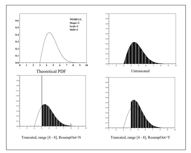
Figure 3.14. The Weibull Distribution in APEX
