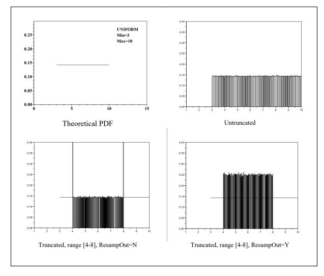
Figure 3.13. The Uniform Distribution in APEX
