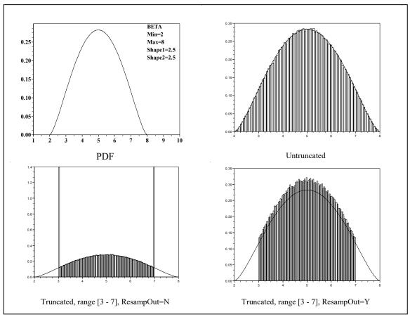
Figure 3.1. The Beta Distribution in APEX
