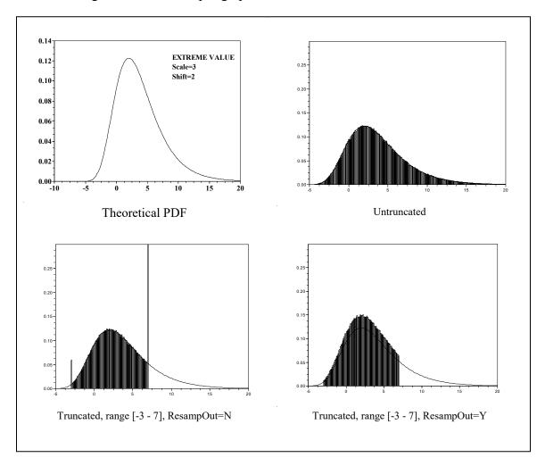
Figure 3.5. The Extreme Value Distribution in APEX
