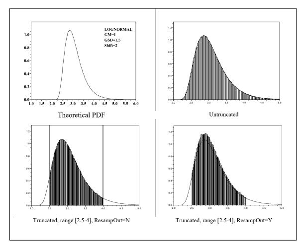
Figure 3.8. The Lognormal Distribution in APEX
