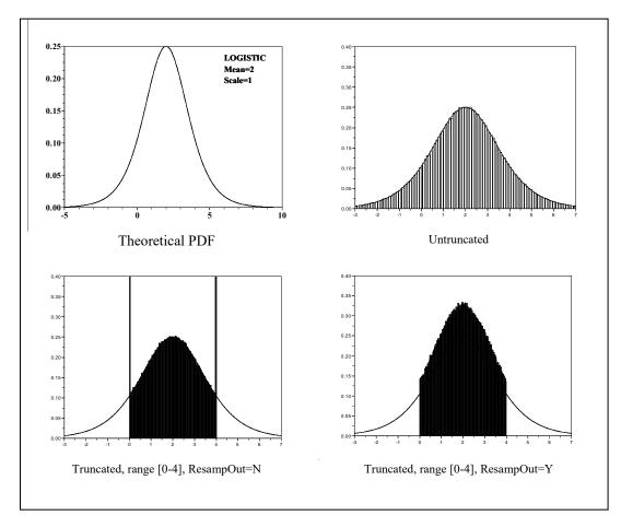
Figure 3.7. The Logistic Distribution in APEX
