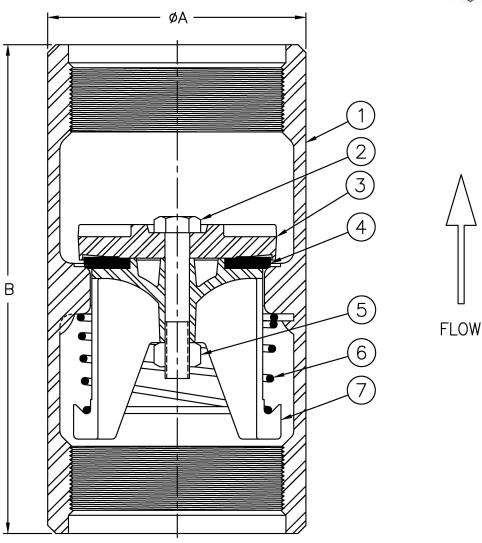
Max Temp 400°F (200°C) Max Pressure 400psi (28bar)
