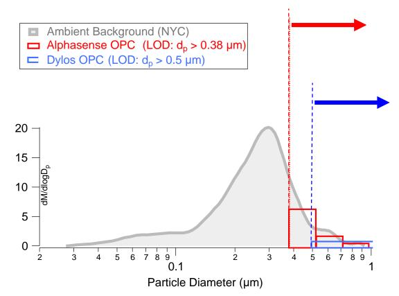
Variability in the size distribution of ambient particulate matter changes the fraction of suspended PM detected by the lowcost OPC
