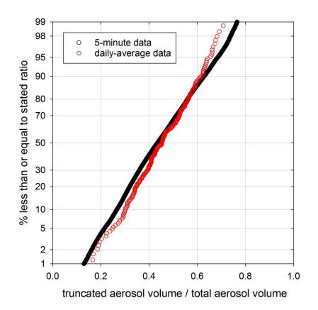
Scaling the truncated (>0.35 μm) aerosol volume to the total aerosol volume
