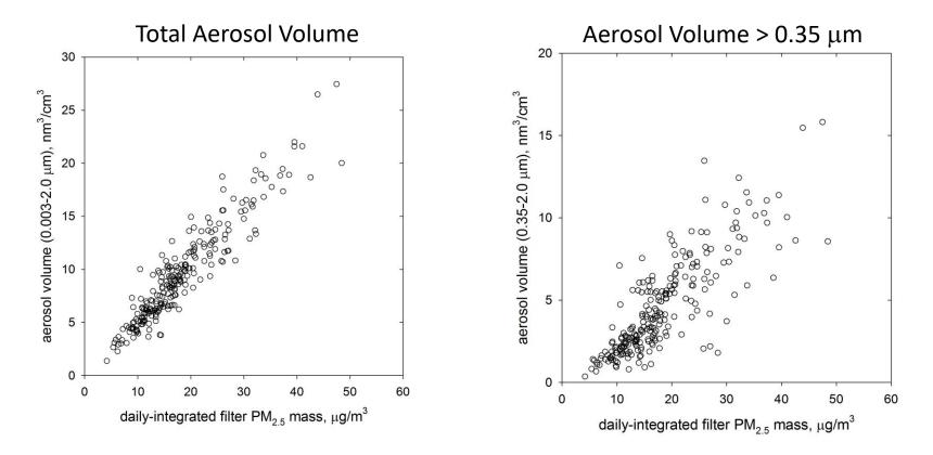
Truncating the PSD to measure only particles larger than 0.35  $\mu$ m leads to much greater variability in the PSD volume – to – gravimetric mass relationship.
