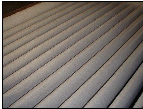
Figure 2-1. Closeup of a Chrysotile Diaphragm Outside of the Electrolytic Cell Photograph courtesy of the American Chemistry Council
