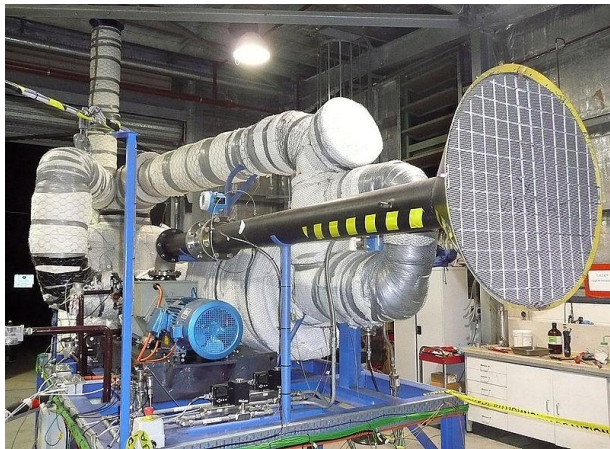
Ventilation Air Methane Catalytic Turbine that traps fugitive methane from the exhaust ventilation air of underground coal mines. Photo Credit: CSIRO
