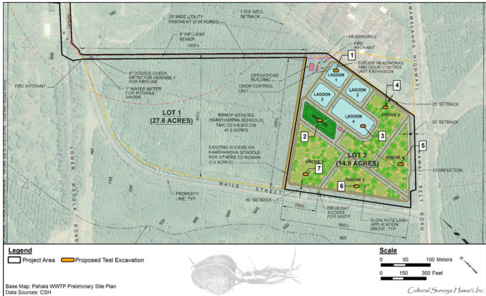
Figure 2. Pahala WWTP Preliminary Site Plan showing AIS test excavation locations
