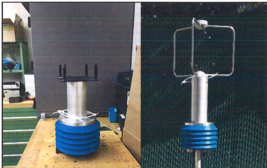
Figure 2: 2D sonic anemometer SPod (left), 3D sonic anemometer (right)
