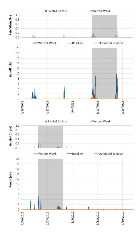
Figure 13. Selected periods of rainfall and runoff for outfall #2 during 2012, a year representing an average amount of precipitation for Tisbury, MA.
