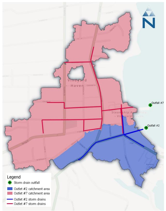
Figure 3.Storm drains, outfalls, and catchment areas
