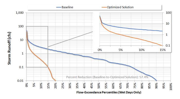
Figure 14. Opti-Tool derived flow duration curves for outfall #2
