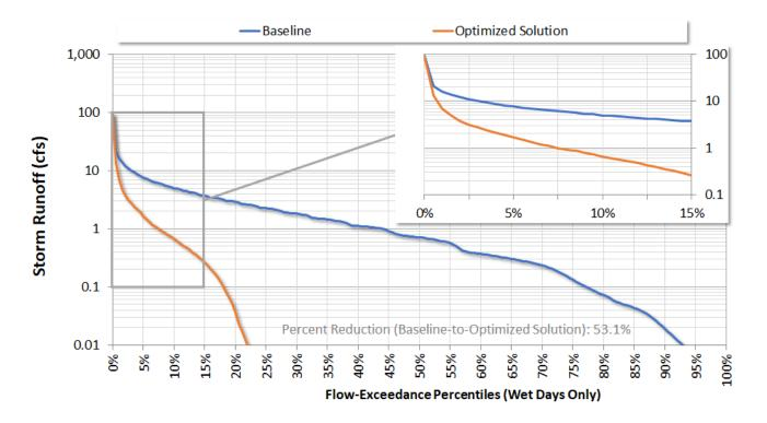
Figure 9. Opti-Tool derived flow duration curves (wet days only) for outfall #7
