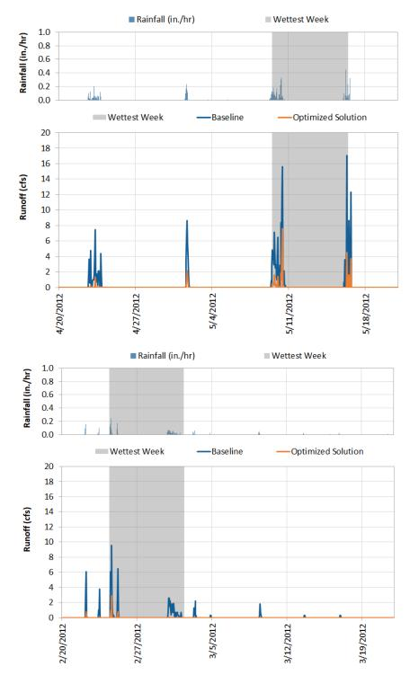
Figure 8. Selected periods of rainfall and runoff for outfall #7 during 2012, a year representing an average amount of precipitation for Tisbury, MA. Grey area highlights the wettest week for the time period shown.
