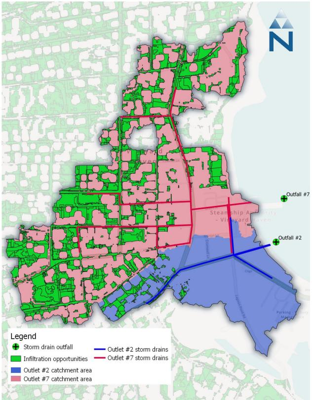
Figure 5. Infiltration-based GI SCM opportunities in the two outfall catchments.
