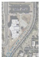
The easement off 16th street includes a bioswale to intercept regional stormwater coming north from South Mountain and prevent it from flooding the schoolyard.
