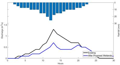
Figure 9. Flow hydrograph at the main channel inlet (point A in Figure 7) for the 2050 NOAA SLR projections with and without the implementation of the proposed wetlands.
