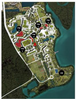
Figure 7. Proposed new wetlands. PW1, PW2, PW3, PW4, PW5 are permeable wetlands for infiltration and pollutant treatment. LW is a lined wetland for stormwater storage for irrigation purposes.
