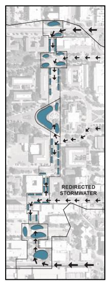
*Fig.* 6 - Basin locations and stormwater movement in Phase I segment of western corridor.
