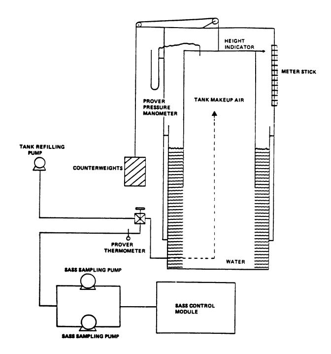
Figure 6. Schematic Diagram of Standard Bell Prover Arrangement for SASS Dry-Gas-Meter Calibration.
