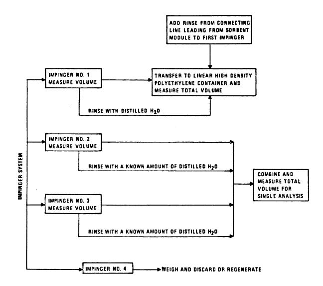
Figure 5. Sample Handling and Transfer Impingers.
