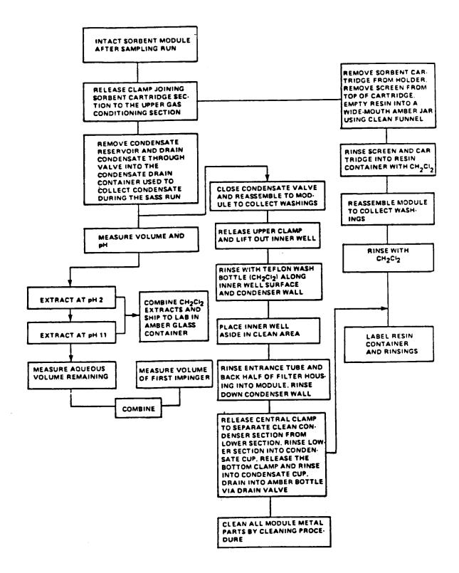
Figure 4. Sample Handling and Transfer XAD-2 Module.
