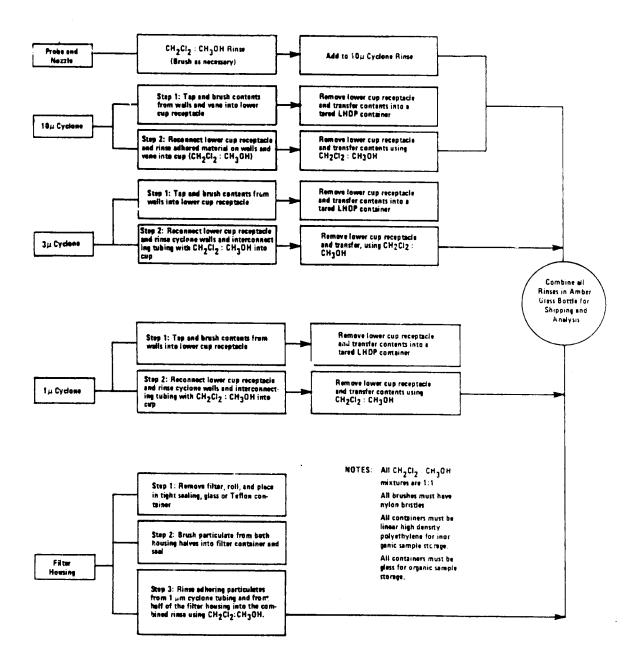
Figure 3. Sample Handling and Transfer Nozzle, Probe, Cyclones and Filter.
