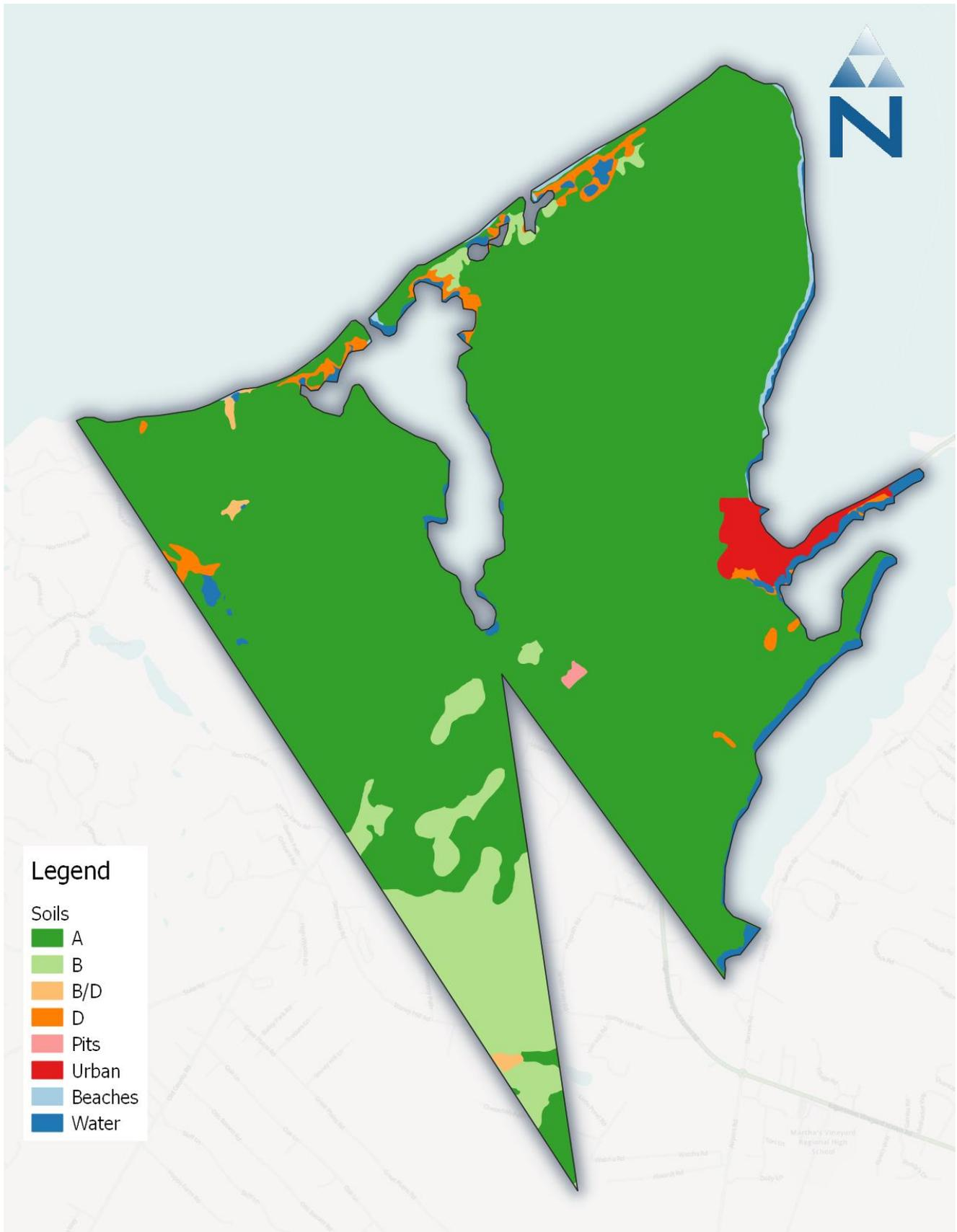
Figure 2-4. Hydrologic soil groups for the Town of Tisbury, MA.
