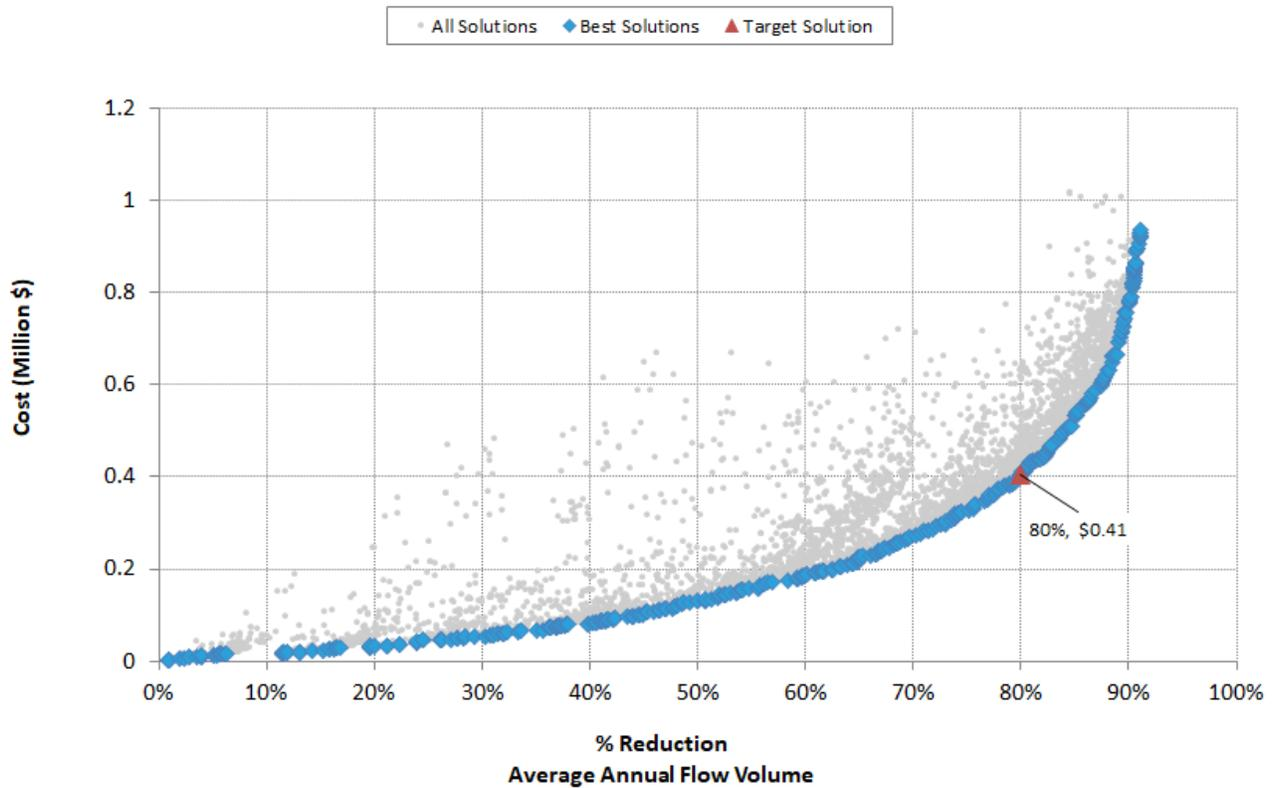
Figure 4-18. Opti-Tool Outfall cost effectiveness curve for annual average flow volume for outfall # 2
