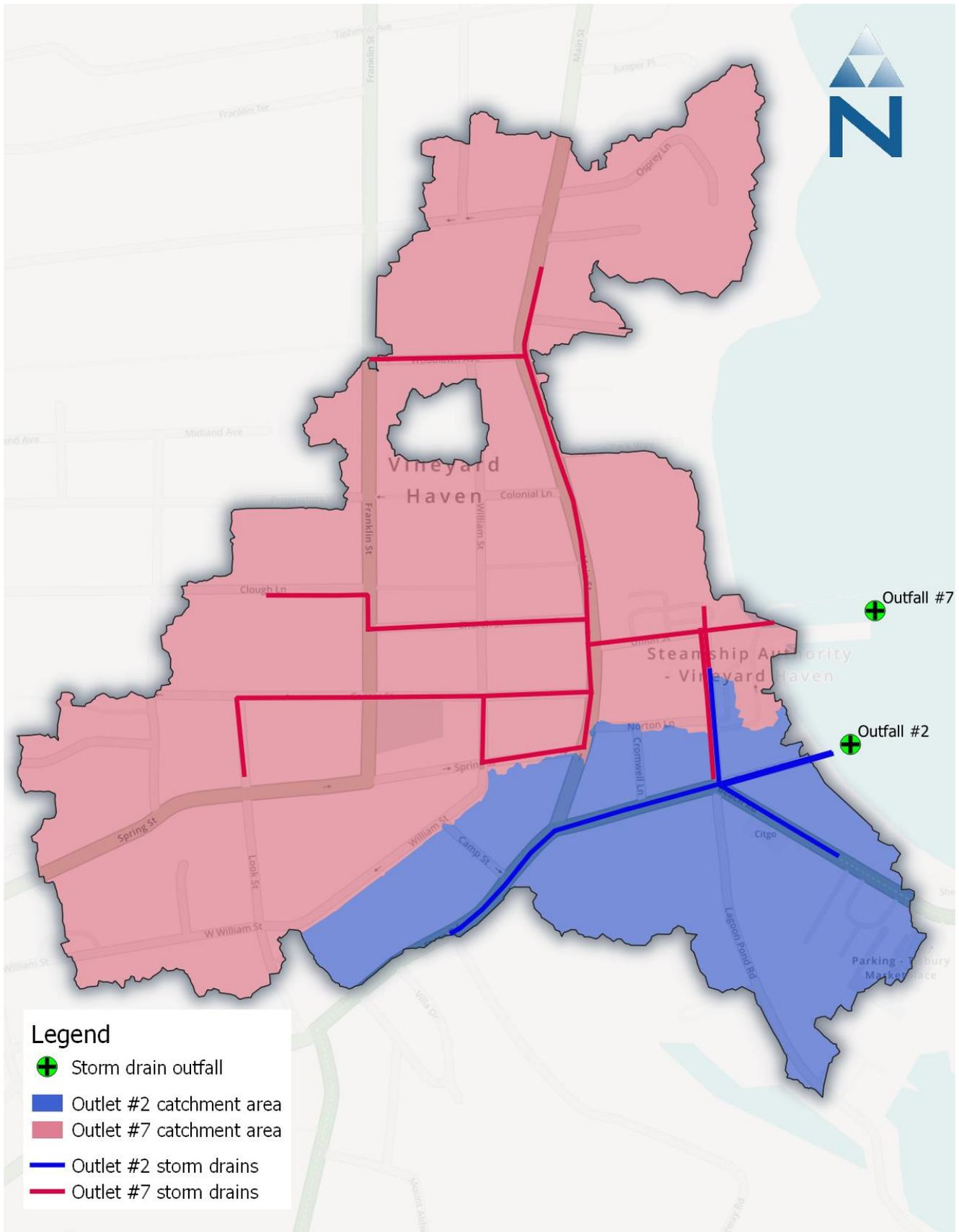
Figure 4-10. Storm drains, outfalls, and catchment areas
