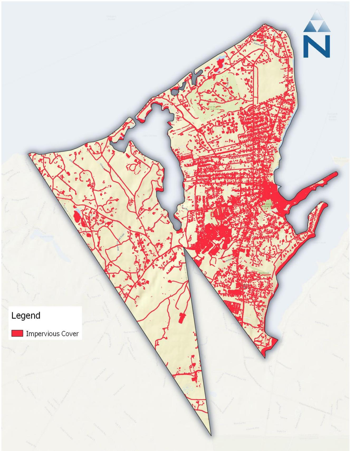
Figure 2-6. Mapped impervious cover for the Town of Tisbury, MA.
