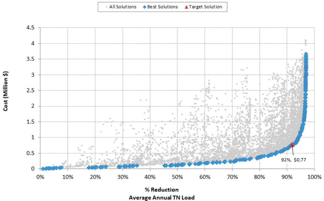
Figure 4-17. Opti-Tool cost effectiveness curve for TN annual average load reduction for outfall #7
