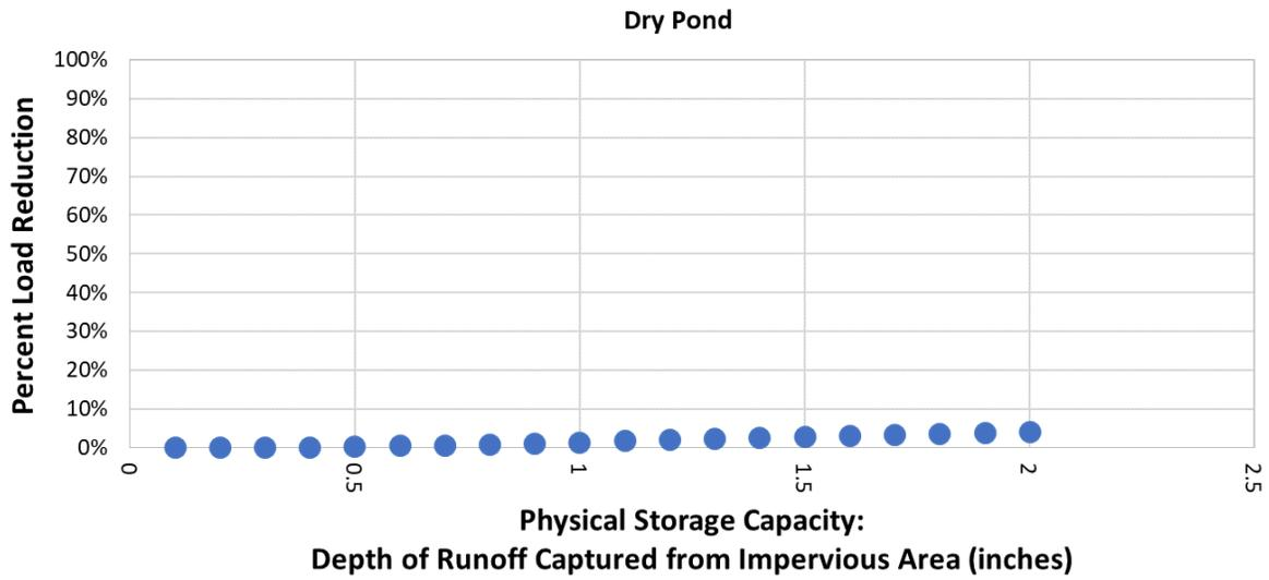
Figure 4-8. Dry Pond performance curve for annual average E. coli load reduction.
