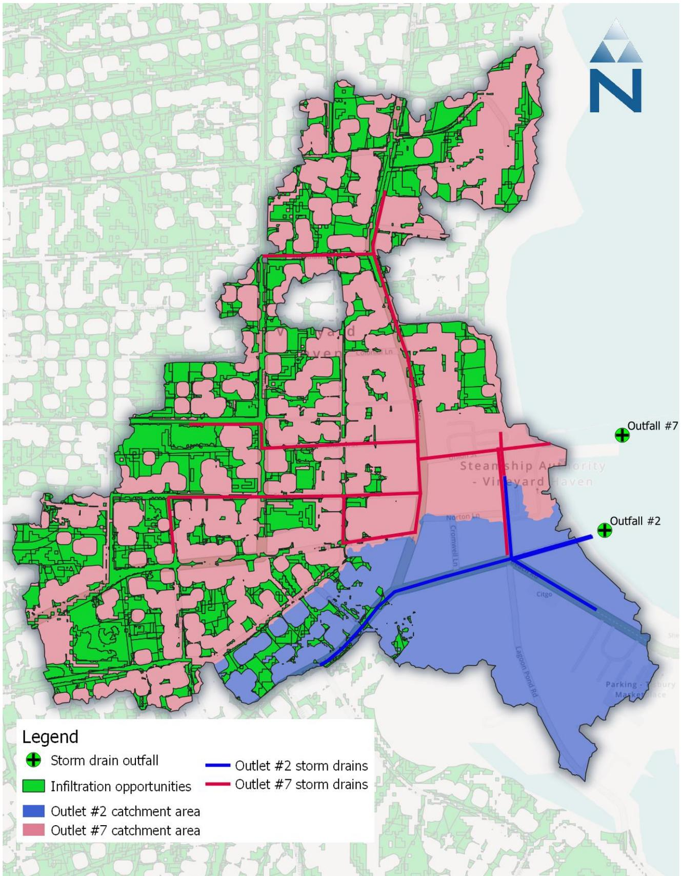
Figure 4-12. Infiltration-based GI SCM opportunities in the two outfall catchments.
