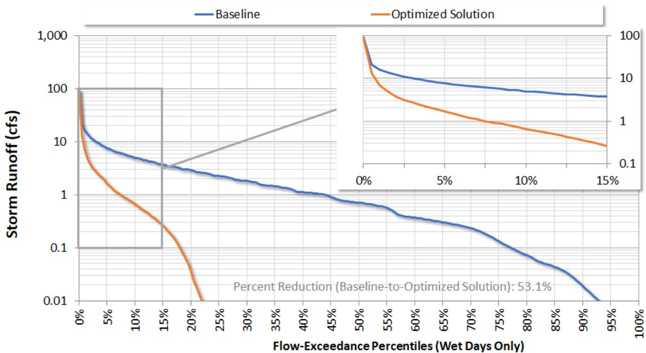
Figure 4-16. Opti-Tool derived flow duration curves (wet days only) for outfall #7
