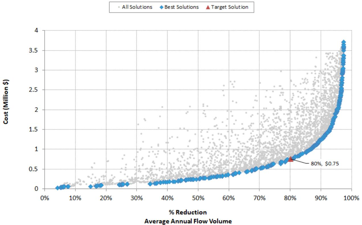
Figure 4-13. Opti-Tool Outfall cost effectiveness curve for annual average flow volume for outfall #7
