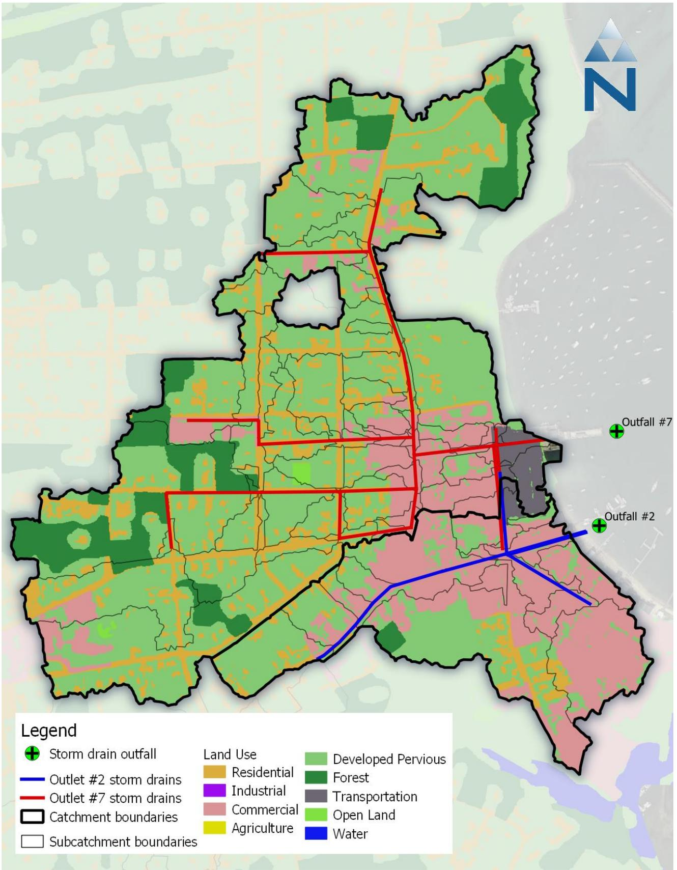
Figure 4-11. Sub-catchment delineation and major land use in the drainage areas to outfall #2 and #7.
