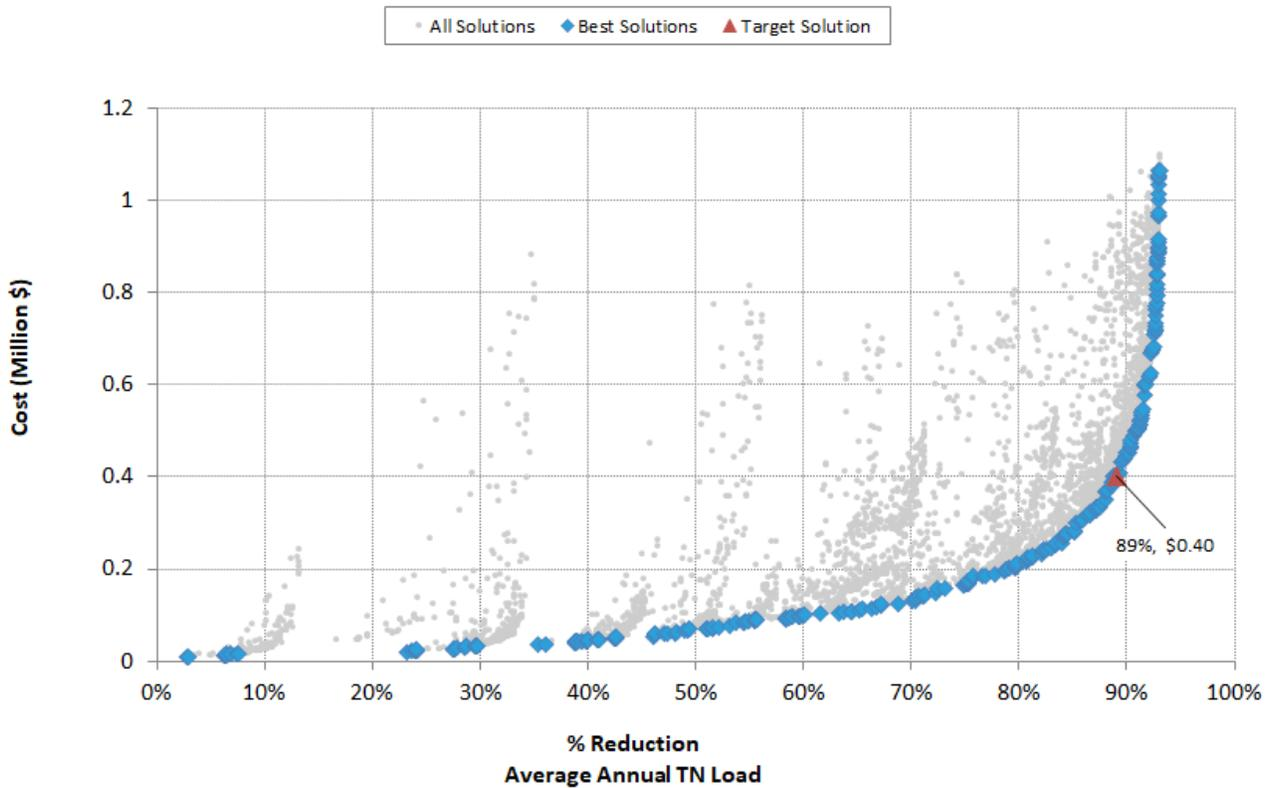
Figure 4-22. Opti-Tool Outfall cost effectiveness curve for TN annual average load reduction for outfall #2
