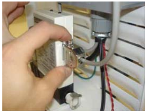
Figure 9.11 Removing MFC Data Cable
