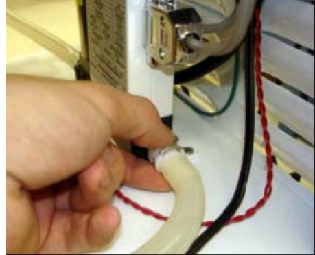
Figure 9.9 Removing Front Hose on to MFC
