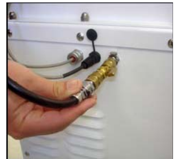
Figure 5.10 Connection of Air Line to Pump Shutoff Valve
