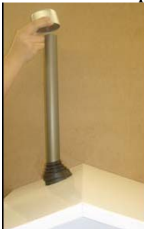
Figure 5.6 Removal of Ambient Air Inlet Cap
