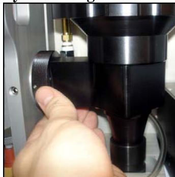
Figure 9.20 Unscrewing the Cyclone Ring
