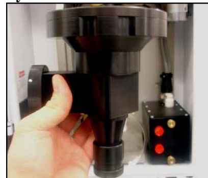
Figure 9.21 Removing the Cyclone
