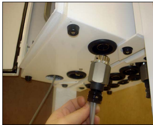
Figure 9.5 Removing the Controller Cable
