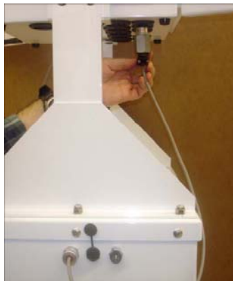
Figure C.18 Side View of Pump Relay Cable Connection
