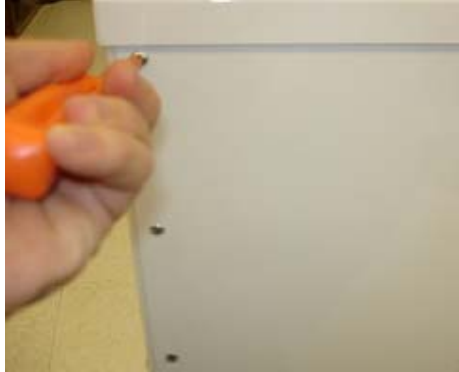
Figure 9.8 Removing the Panel Pump Enclosure
