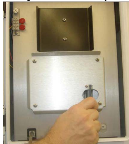
Figure C.28 Inserting the Compact Flash Memory Card
