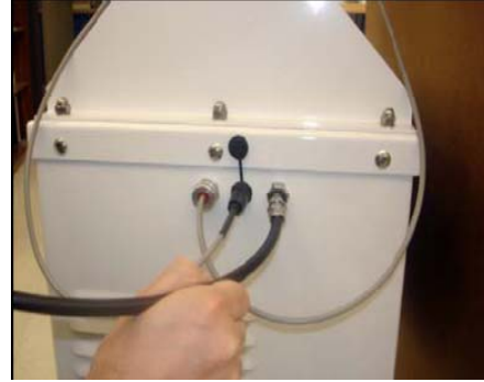
Figure C.24 Connection of Air Line to the Lower Stand (Pump Enclosure)
