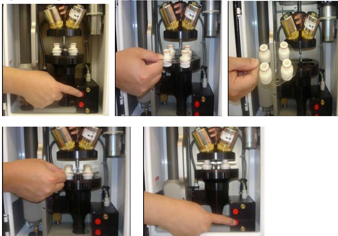
Figure 5.2 Replacement of Sample Cartridge with AUDIT Cartridge
