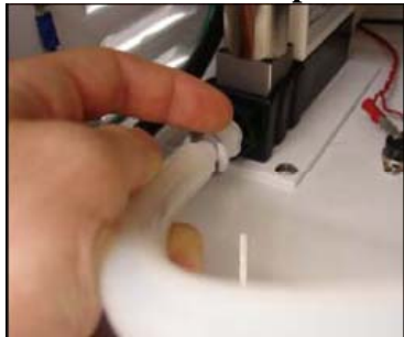
Figure 9.15 Disconnect Hose From MFC to Pump
