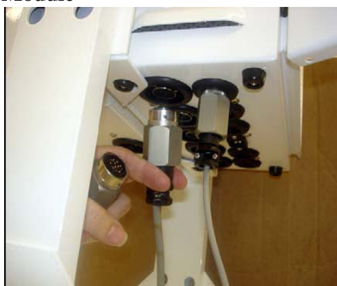
Figure C.20 Connection of the Controller Cable to Controller Module
