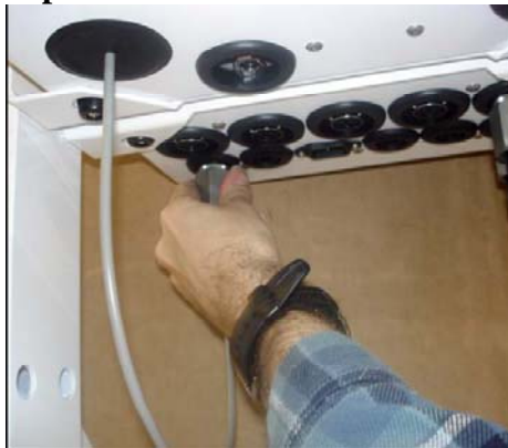
Figure C.25 Connection of the Ambient Temperature Probe to the Sample Module and Controller Module
