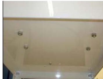
Figure 9.14 Remove Nuts from Bottom of Pump Enclosure
