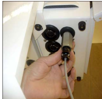
Figure C.19 Connection of the Pump Relay Cable to bottom of Controller Module
