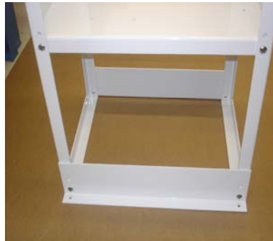
Figures C.10 to C.12 Installing of the Upright Support to the Base and the Proper Installation of the Support Feet
