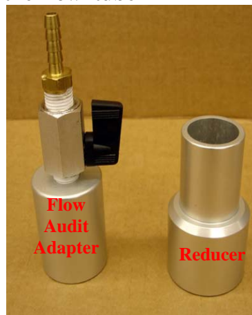
Figure 5.7 Placing the Reducer and the Flow Audit Adapter on the Downtube
