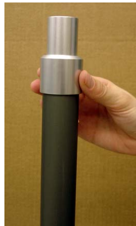
Figure 5.7 Placing the Reducer and the Flow Audit Adapter on the Downtube
