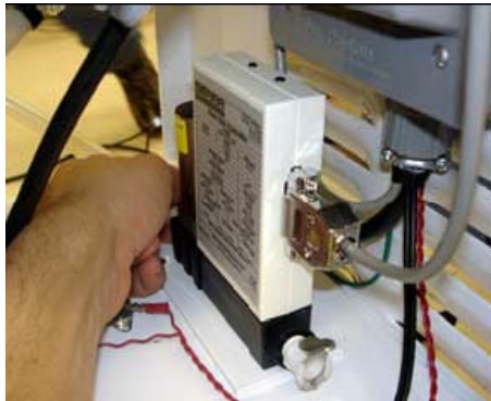
Figure 9.10 Removing Rear Hose to MFC
