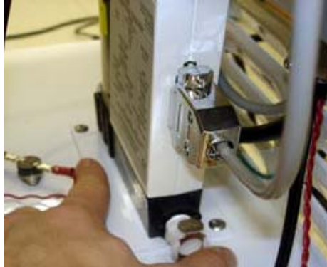
Figure 9.12 Removing MFC and Base Plate
