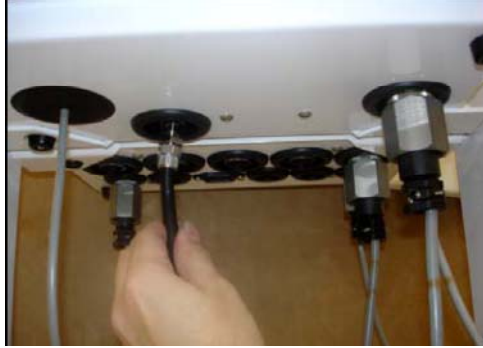
Figure C.23 Connection of Air Line to the Sample Module
