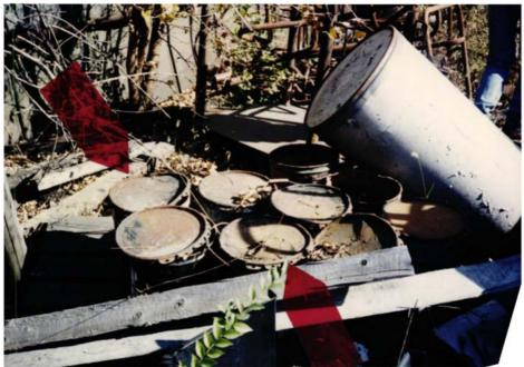
9 pails of unknown about 6ft to east of sample point 001. The two pails pointed out by the red arrows measured 9 units on the Hnu meter (10.2eV probe). All others measured no detection D. Newsome
