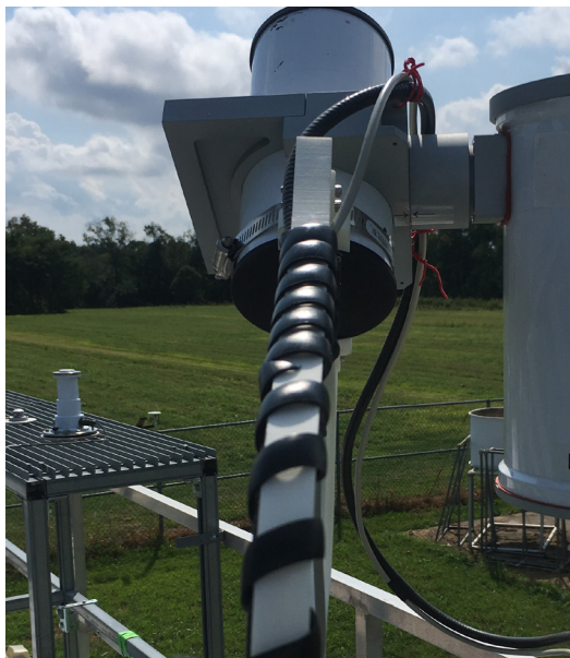
A ground-based Pandora spectrometer for satellite validation on the New Jersey Department of Environmental Protection air quality monitoring site at Rutgers University in New Brunswick, NJ.
