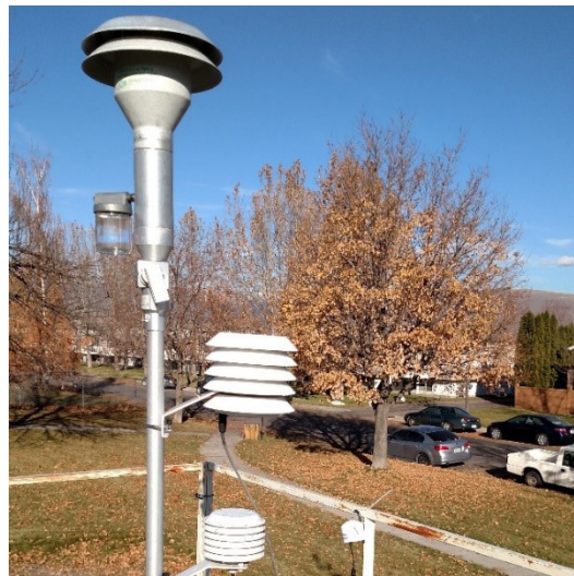
Air sensors operating in close proximity to regulatory-grade or other conventional air quality monitors in Iowa.
