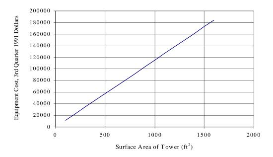
Figure 1.7: Packed Tower Equipment Cost [16]
