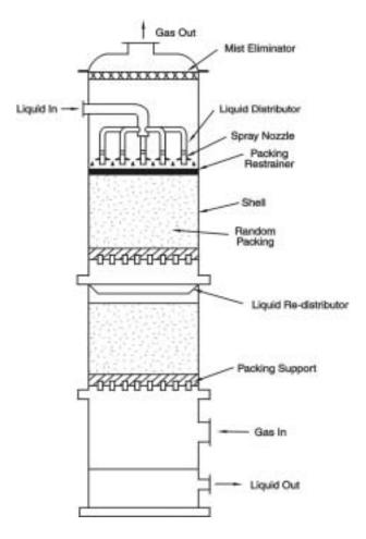
Figure 1.1: Packed Tower for Gas Absorption
