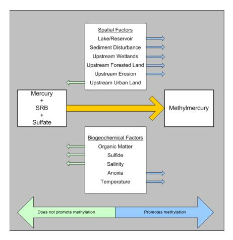
**Figure 4-1. Spatial and Biogeochemical Factors Influencing MeHg Production** and MeHg could not be quantified for the purpose of interpolating the association across waterbodies or regions. Nevertheless, because changes in MeHg in ecosystems represent changes in significant human and ecological health risks, the association between sulfur and mercury cannot be neglected (EPA, 2008, Sections 4.4.1 and 4.5).
