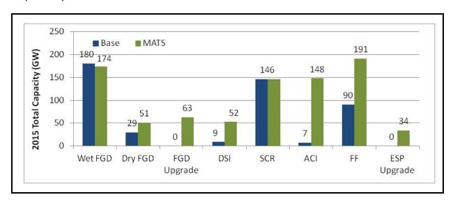
Figure 3-6. Operating Pollution Control Capacity on Coal-fired Capacity (by Technology) with the Base Case and with MATS, 2015 (GW)
