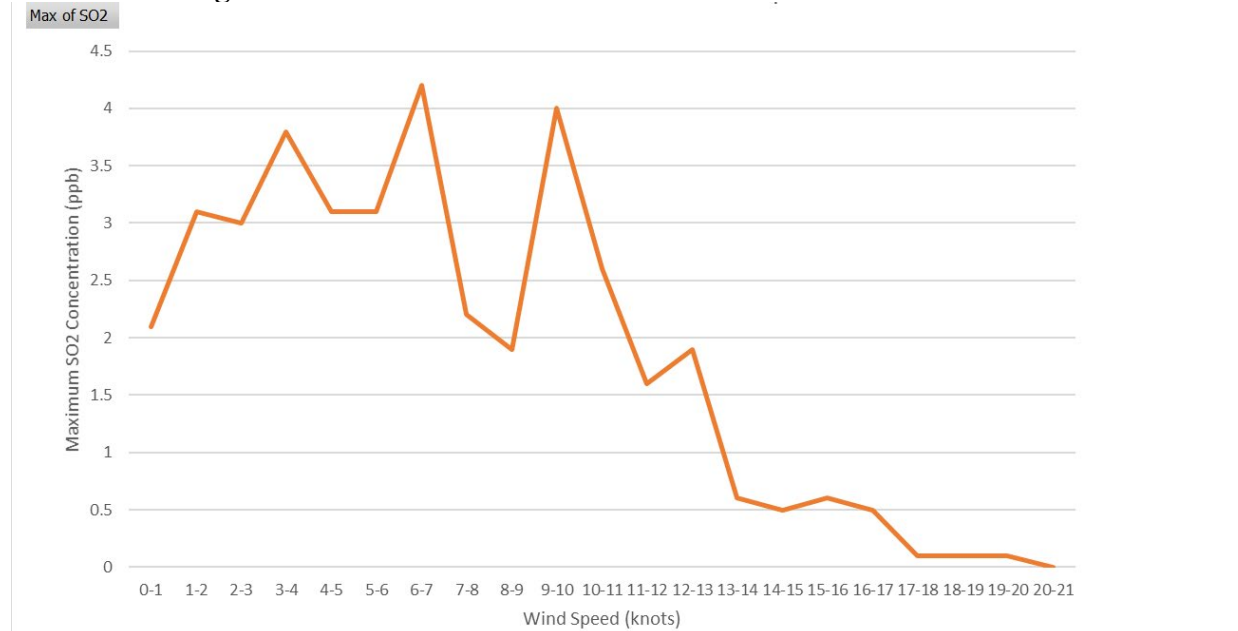
Figure 33. Relationship of Maximum SO 2 Concentration Versus Wind Speed at the DRR Monitor During 2019 for All Wind Directions.
