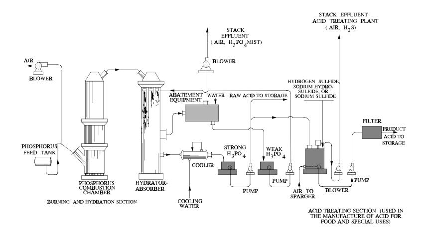
Figure 8.9-2. Flow diagram of a thermal process phosphoric acid plant.
