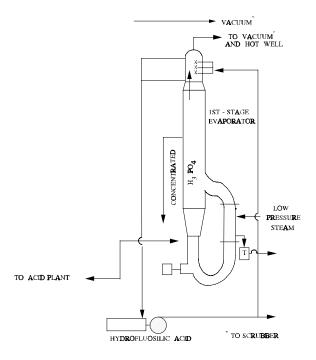
Figure 8.9-1B. Flow diagram of a wet process phosphoric acid plant (cont.).
