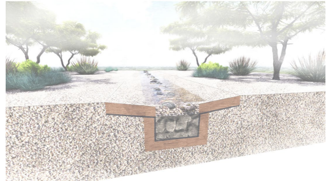
Figure 1: Illustration of an infiltration trench (Source: Flood Control District of Maricopa County. Reduce Your Flood Risk: A Resource Guide . June 2019.)
