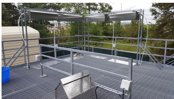
Figure 2. PE Sampling system consisting of 32 PM 2.5 cyclones on four sampling manifolds and one dedicated pump (in fancy pump-box in the foreground)
