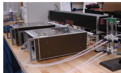
SRP verifying transfer standards
