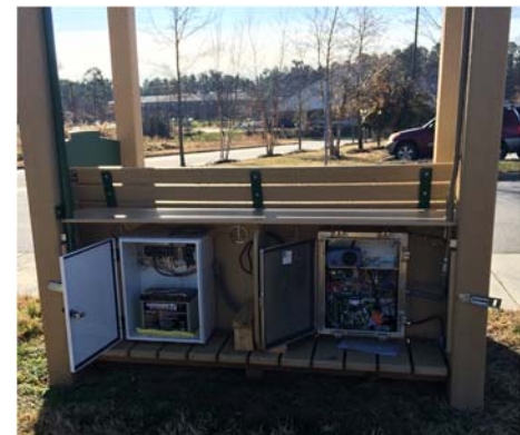
Ozone and PM monitors behind the bench
