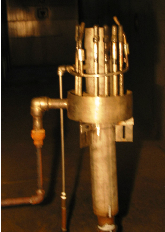
Figure 2 - Photo of steam ring with pilot burners
