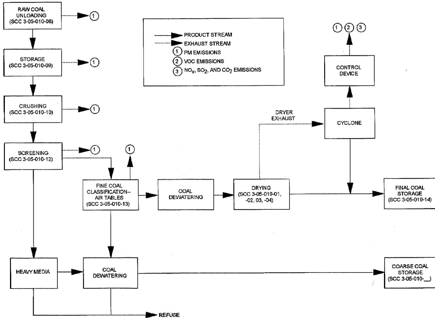
Figure 2-1. Typical coal cleaning plant process flow diagram.
