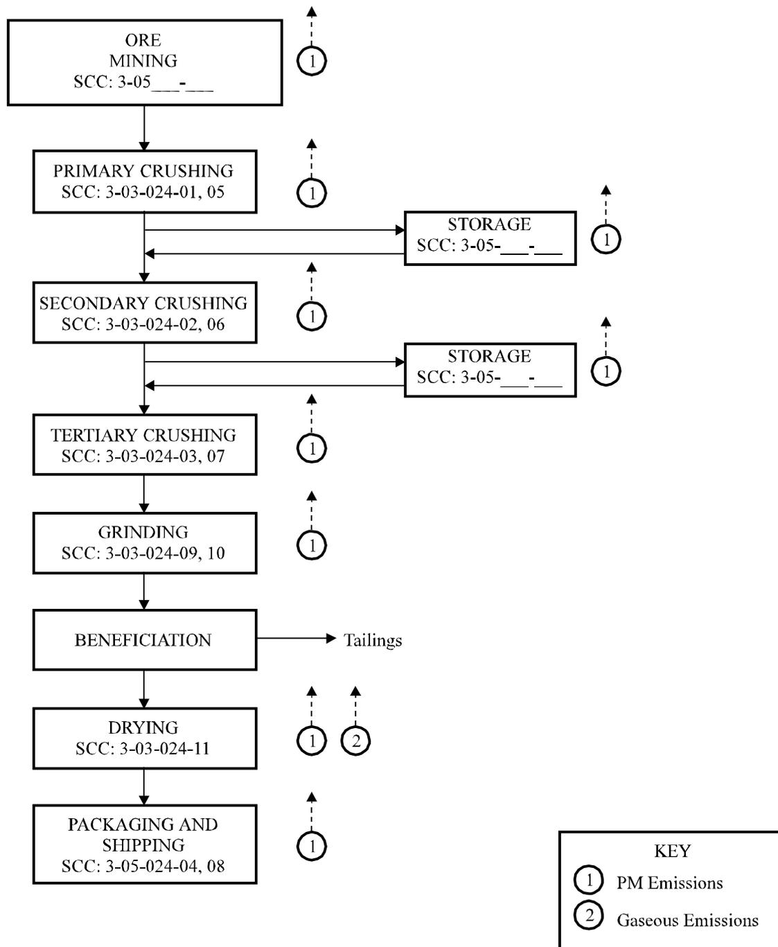
Figure 11.24-1. Process flow diagram for metallic mineral processing.
