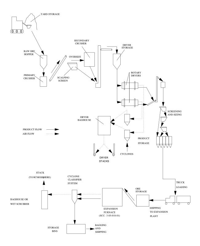
Figure 11.30-1. Flow diagram for perlite processing.<sup>1</sup> (Source Classification Code in parentheses.)
