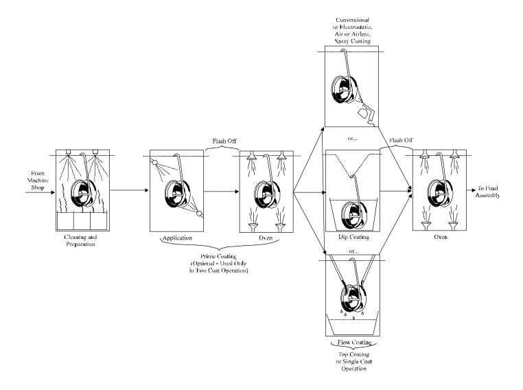
Figure 4.2.2.4-1. Metal product coating line emission points.
