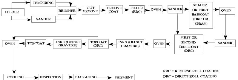
Figure 4.2.2.5-1. Flat wood interior panel coating line emission points.
