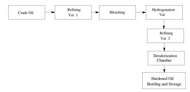
Figure 9.13.1-4. Oil hardening process.
