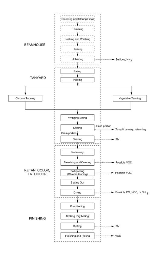
Figure 9.15-1. General flow diagram for leather tanning and finishing process.
