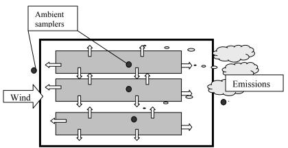
**FIGURE 4-5.** Schematic illustrating the essential elements associated with the regulation of emissions from agricultural sources that can be characterized as low-level point sources such as naturally ventilated AFOs.
