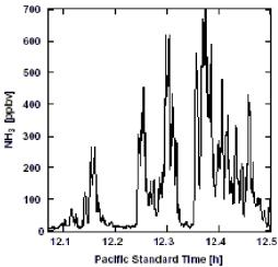
**FIGURE 4-1.** Ammonia concentrations (averaged over a 68-m path) measured near a dairy wastewater lagoon. Method used was an ultraviolet differential optical absorption spectroscopy technique with a detectability limit of 1 ppb and a time resolution of 0.6 second. SOURCE: Reprinted from Mount et al., 2002, with permission from Elsevier Science.
