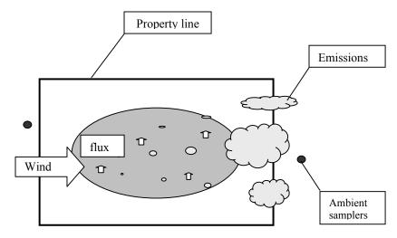
**FIGURE 4-3.** Schematic illustrating the essential elements associated with measurement of emissions from agricultural sources that can be characterized as ground-level area sources such as dairies, cattle feed yards, field operations, and agricultural burning.
