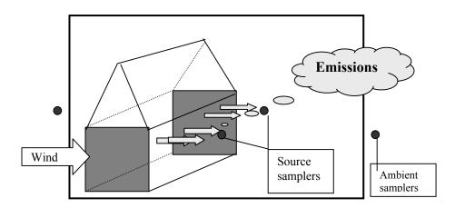
**FIGURE 4-2.** Schematic illustrating the essential elements associated with measurement of emissions from agricultural sources that can be characterized as low-level point sources such as cotton gins, feed mills, grain elevators, and oil mills.
