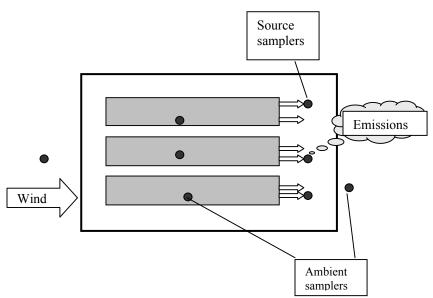
**FIGURE 4-4.** Schematic illustrating the essential elements associated with the regulation of emissions from agricultural sources that can be characterized as low-level point sources such as tunnel-ventilated AFOs.
