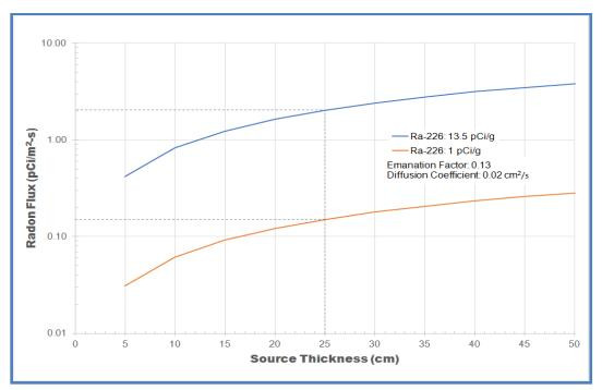
Figure 4-9 SC&A Calculated Effect of Source Thickness on Radon Surface Flux
