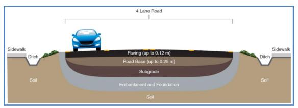
Figure 4-1 Schematic Cross-Section of the Road Modeled by Arcadis 2019 (Source: TFI 2019, Appendix 1, Figure S-1)
