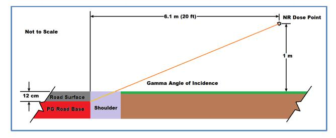
Figure 4-3 Schematic of the After Construction, Nearest Resident Exposure Pathway
