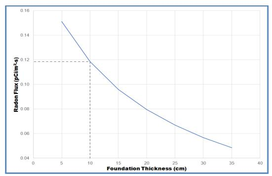
Figure 4-10 SC&A Calculated Radon Flux Through the Foundation with a 6-mm Poly Vapour Barrier
