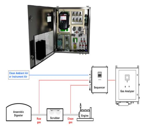
Figure 7-1. Gas analyzer and flow diagram of sequence and gas analyzer.
