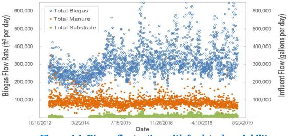
Figure 4-1. Biogas fluctuation with feedstock variability.<sup>6</sup>
