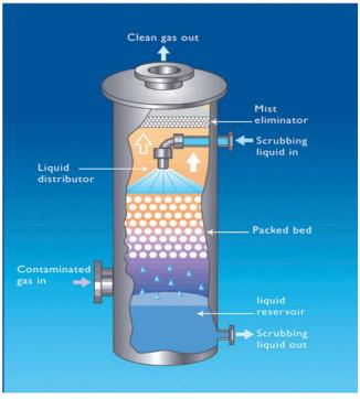
Figure 7-4. Cross-section of a packed tower scrubber for an H<sub>2</sub>S removal system. <sup>19</sup>
