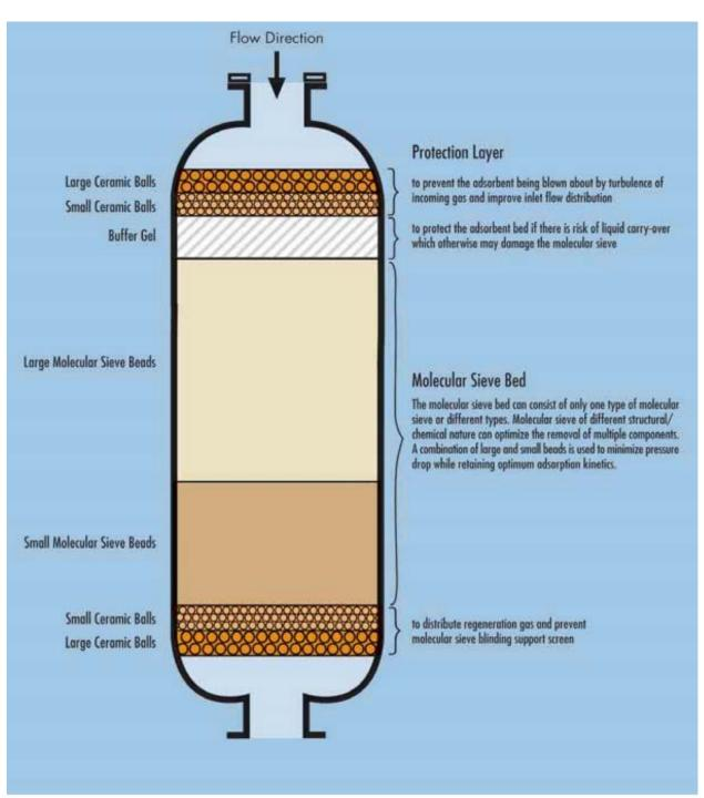
Figure 7-5. Cross-section of a typical adsorber bed.<sup>20</sup>
