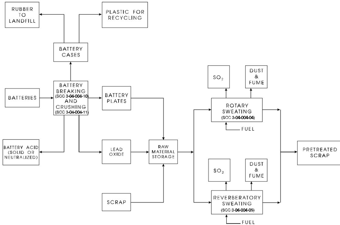
Figure 12.11-1A. Process flow for typical secondary lead smelting.
