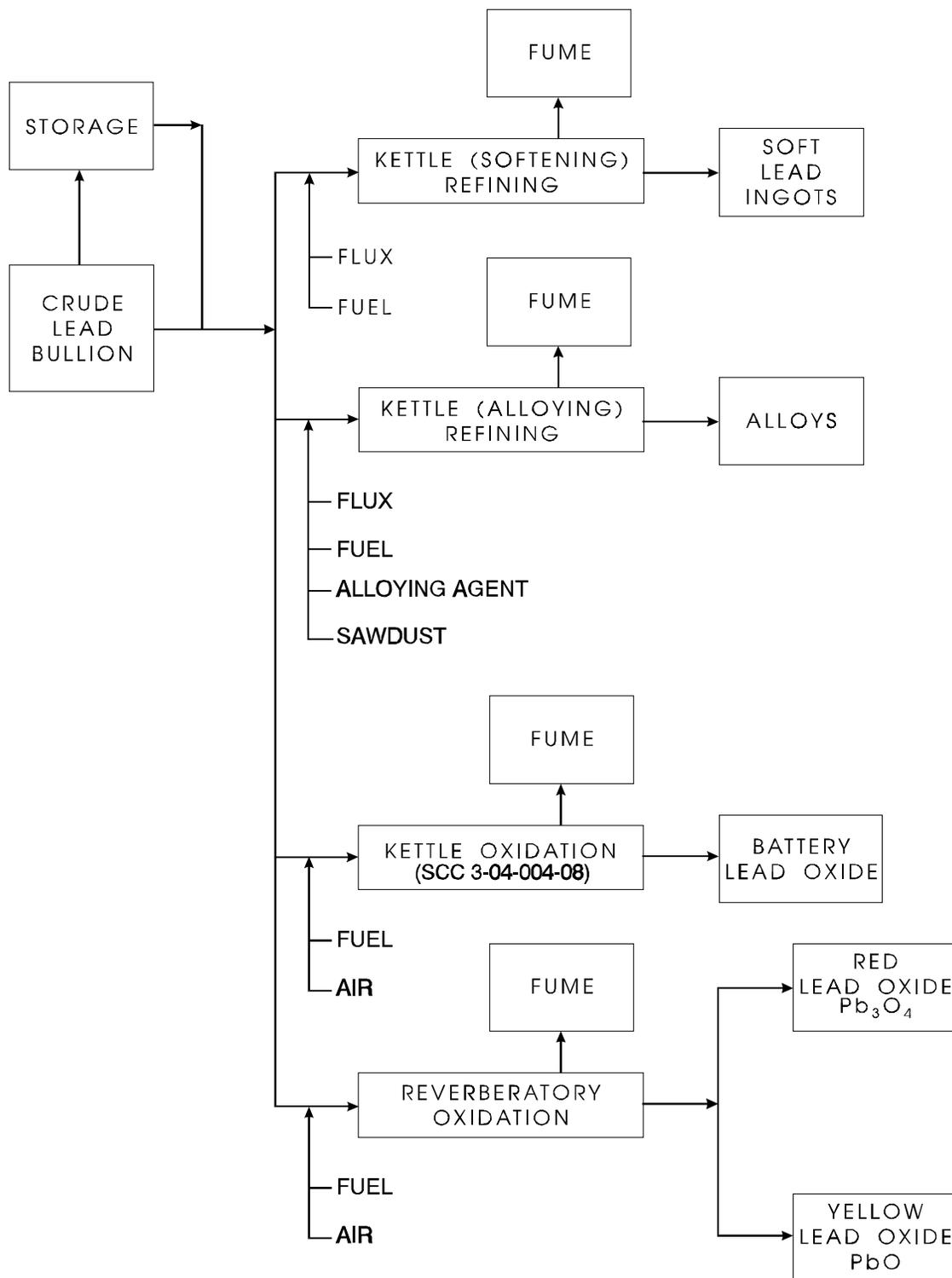
Figure 12.11-1C. Process flow for typical secondary lead smelting.
