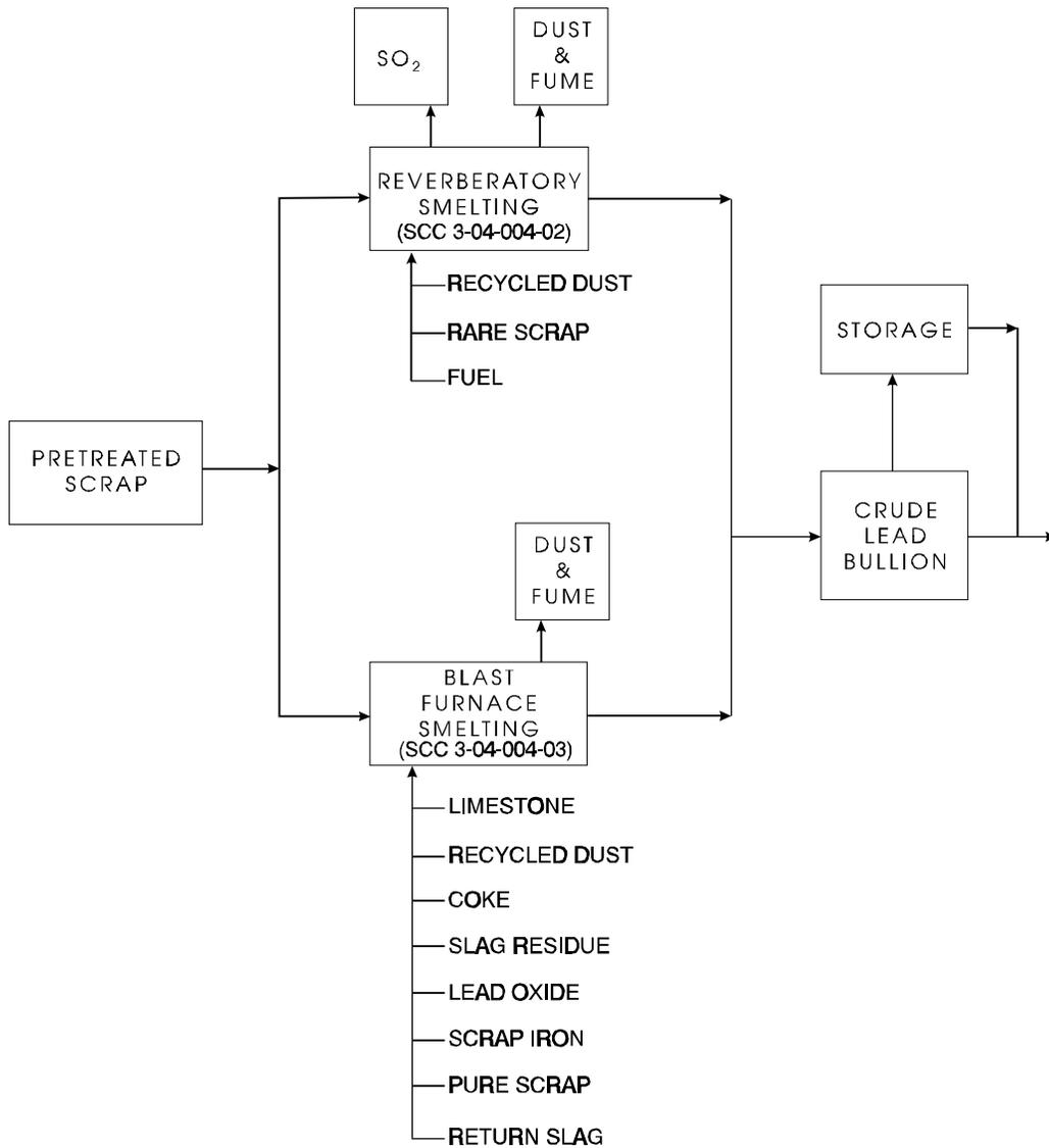
Figure 12.11-1B. Process flow for typical secondary lead smelting.
