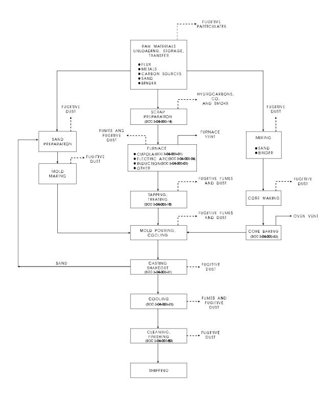
Figure 12.13-1. Flow diagram of a typical steel foundry. (Source Classification Codes in parentheses.)
