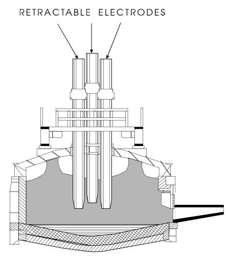
Figure 12.13-2. Electric arc steel furnace.
