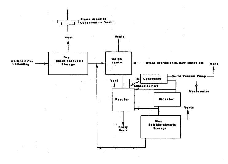
Figure 4. Flow diagram for the batch production of epoxy resins.<sup>11</sup>
