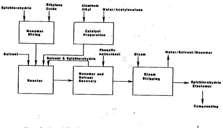
Figure 5. General flowsheet for the production of epichlorohydrin elastomers.<sup>1</sup>
