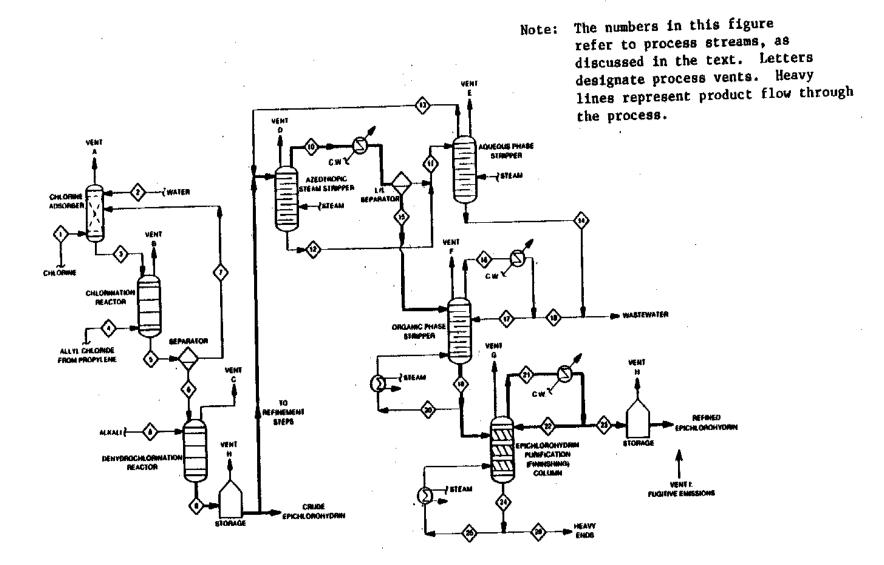
Figure 1. Basic Operations that May Be Used in the Production of Epichlorohydrin from Allyl Chloride
