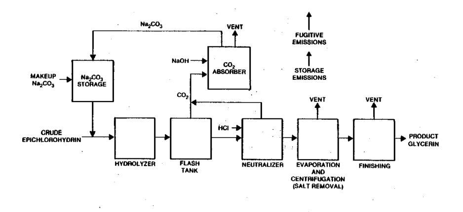
Figure 2. Basic operations that may be used in the production of synthetic glycerin from epichlorohydrin.
