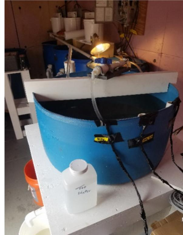
*Testing to develop a low-cost sensor to record nitrogen concentration in effluent released from innovative/ alternative septic systems. Location: Massachusetts Alternative Septic System Test Center*
