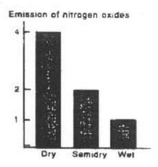
The investigation showed that the three different cutting techniques gave a constant ratio between the amount of emitted fumes of 100:10:1 (dry = 100, semidry = 10, wet = 1). Similarly there was a constant ratio between the amount of emitted nitrogen oxides of 4:2:1 for dry, semidry and wet cutting. These relationships are valid both for mild and stainless steel.
