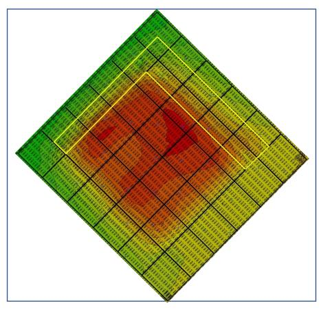
**Figure 4: Open disposal cells at HOODS for 2020** are outlined by the bright yellow box. Black grid depicts the same disposal cells as shown on Figure 3. Here, disposal cell boundaries are overlain on the most recent (2019) bathymetry with green and yellow shading being deeper areas, and orange and red shading being shallower.
