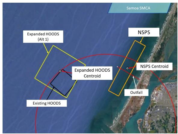
Location of the potential Nearshore Sand Placement Site (NSPS) in relation to the Samoa SMCA, HOODS, and the Fairhaven Power Plant outfall. The red arc is set at the distance (3.7 nmi) from the north jetty to the HOODS center point (centroid), showing that transport distance to much of the NSPS is shorter than to HOODS.
