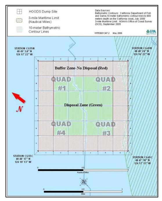
**Figure 4. HOODS Detail.** The site is divided into 4 quadrants and 36 individual cells. Initially, dredged-material disposal was only allowed in the green interior cells, so that material placed at the site would remain largely contained within the overall site.
