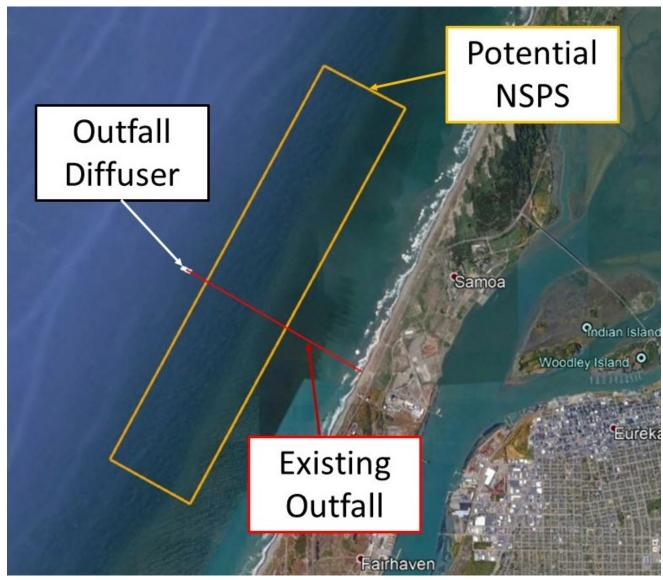
Figure 19. Location of existing outfall relative to the potential Nearshore Sand Placement Site (NSPS).
