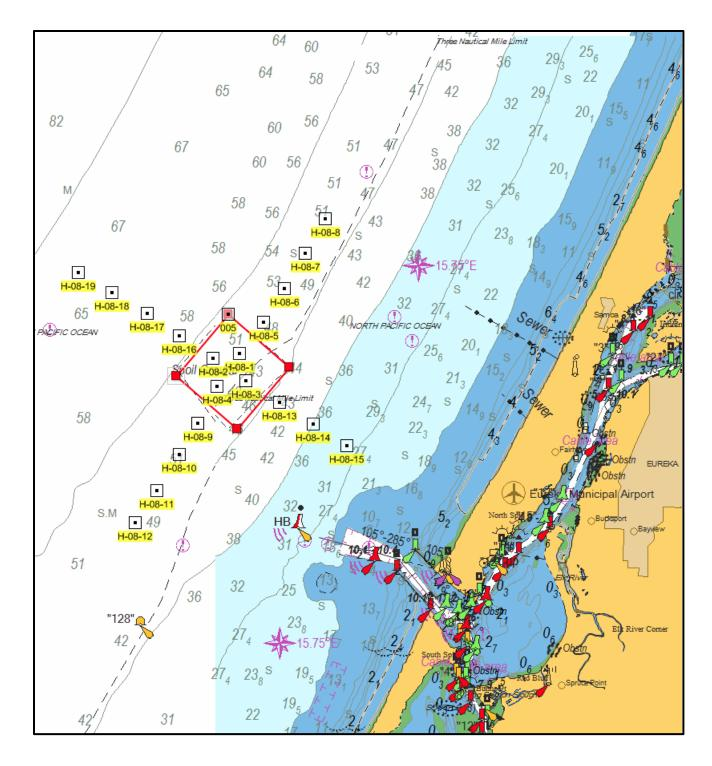
Figure 12. Sediment sampling stations occupied in the 2008 EPA monitoring survey at HOODS. Surface sediment grab samples were obtained from 19 stations (4 inside the site boundary - red box) for physical, chemical, and benthic community analysis. (Mapped on NOAA chart 18620A, 10-19-2009 update; soundings in meters.) (EPA 2016)
