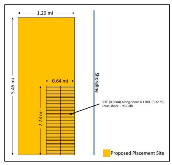
Figure 23. Humboldt Bay Demonstration Site as proposed by USACE in 2012. Cross-hatching shows the Target Placement Area (TPA) recommended at the time for monitored placement of up to 1.5 million cy of sand.
