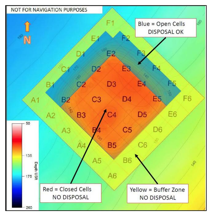
Figure 7. Open and closed disposal cells at HOODS starting in 2015. Disposal only allowed over the north and west slopes of the mound including portions of eight Buffer Zone cells on those sides. This increased short-term disposal capacity by 5.6 - 8 million cy, enough for approximately 5 more years, or through at least 2020.
