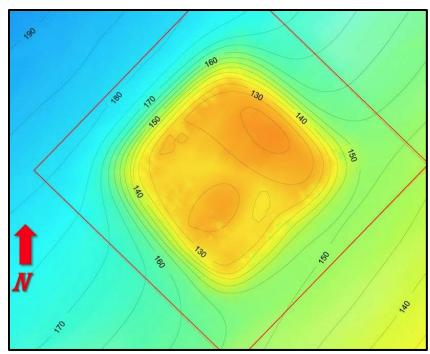
Figure 5. Shaded relief depiction of bathymetry at HOODS as of August 2014, showing mounding to -130 feet or less over much of the site. Red box is the existing disposal site boundary. Contours are in 5-foot intervals. Depths are shown in feet MLLW. (Reproduced from eTrac, 2014.)
