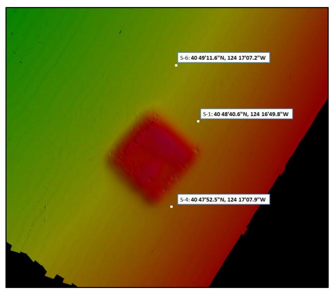
Figure 18. Locations of three "magnetic anomalies" near HOODS. Evaluation of high-resolution data from the 2014 multibeam echosounder survey confirmed that these features, if still present at all, are buried and do not project to or above the sediment surface. (Red shading is the existing HOODS mound.)
