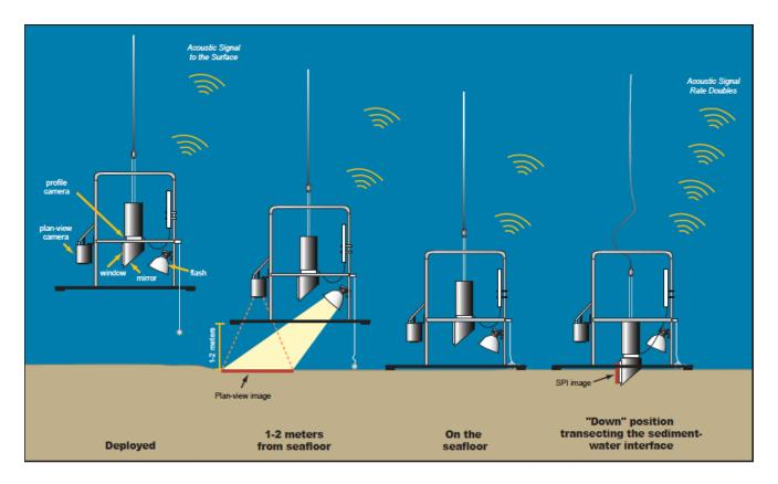
Figure 8. Schematic of deployment and collection of sediment profile images and plan view photographs. (Reproduced from Germano & Assoc., 2014).
