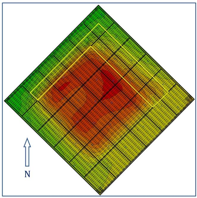
Figure 9: Open disposal cells at HOODS for 2020 are outlined by the bright yellow box. Black grid depicts the same disposal cells as shown on Figure 7. Here, disposal cell boundaries are overlain on the most recent (2019) bathymetry with green and yellow shading being deeper areas, and orange and red shading being shallower.
