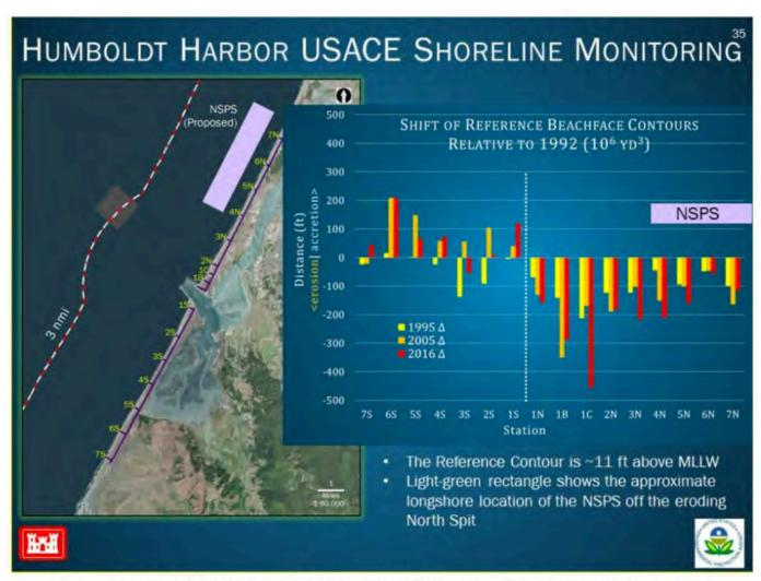
Figure 22. Reference stations and shoreline shifts at selected surveys (1995, 2005, and 2016) relative to the initial survey (1992).
