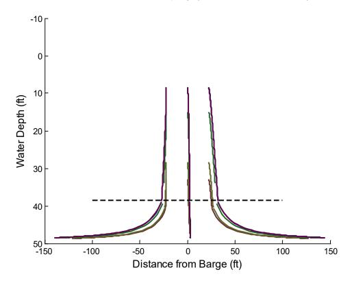
**Trajectory of the dredged sand during placement.** The dashed line represents the collapse zone, or where the material begins to interact with the bed.
