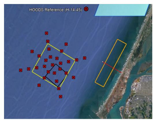
**Figure 9.** Typical sediment sampling station array for periodic site monitoring at HOODS. The expanded HOODS is outlined in yellow, the original HOODS (now closed) is outlined in black, and the potential future Nearshore Sand Placement Site is outlined in orange. The new HOODS reference site is also shown.
