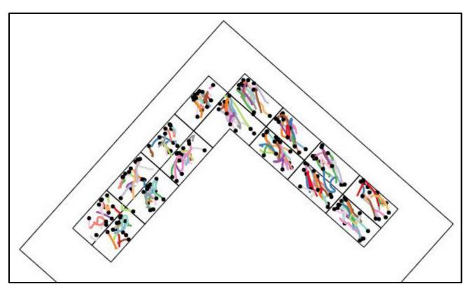
Figure 8. Locations of actual disposal events at HOODS in 2015. All disposal actions occurred successfully within the modified disposal cells, despite most of them being only ½ the size of previously allowed disposal cells. Dots with lines show starting point and track of individual disposal events. (Source: EPA compliance records for USACE 2015 West Coast Hopper contract no. W9127N-15-C-0006).
