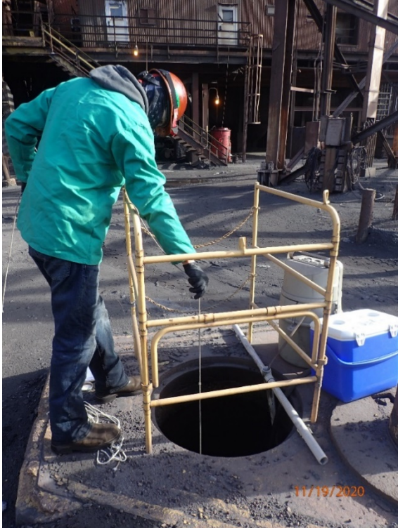
20: PB190020 Description: Taking a sample from sample location #02. Location: Storm Sewer Manhole #2816. Date/Time: November 19, 2020 10:00 A.M.
