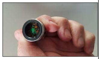
Picture of an aerator with particulate
