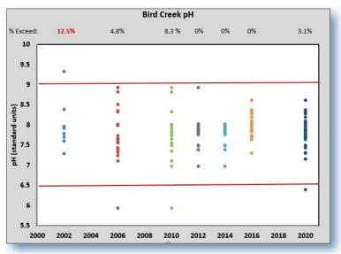
Figure 2. pH levels in Bird Creek improved with installation of CPs.
