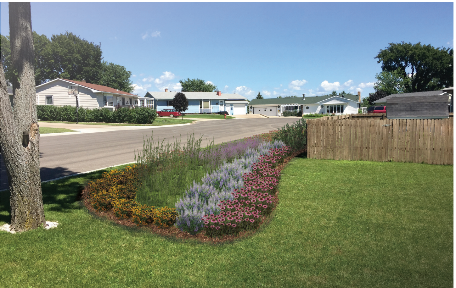
Figure 20: Design concept for the cul-de-sacs at Court A, B and C at Central Avenue North showing a bioswale along the southern edge of Court B.
