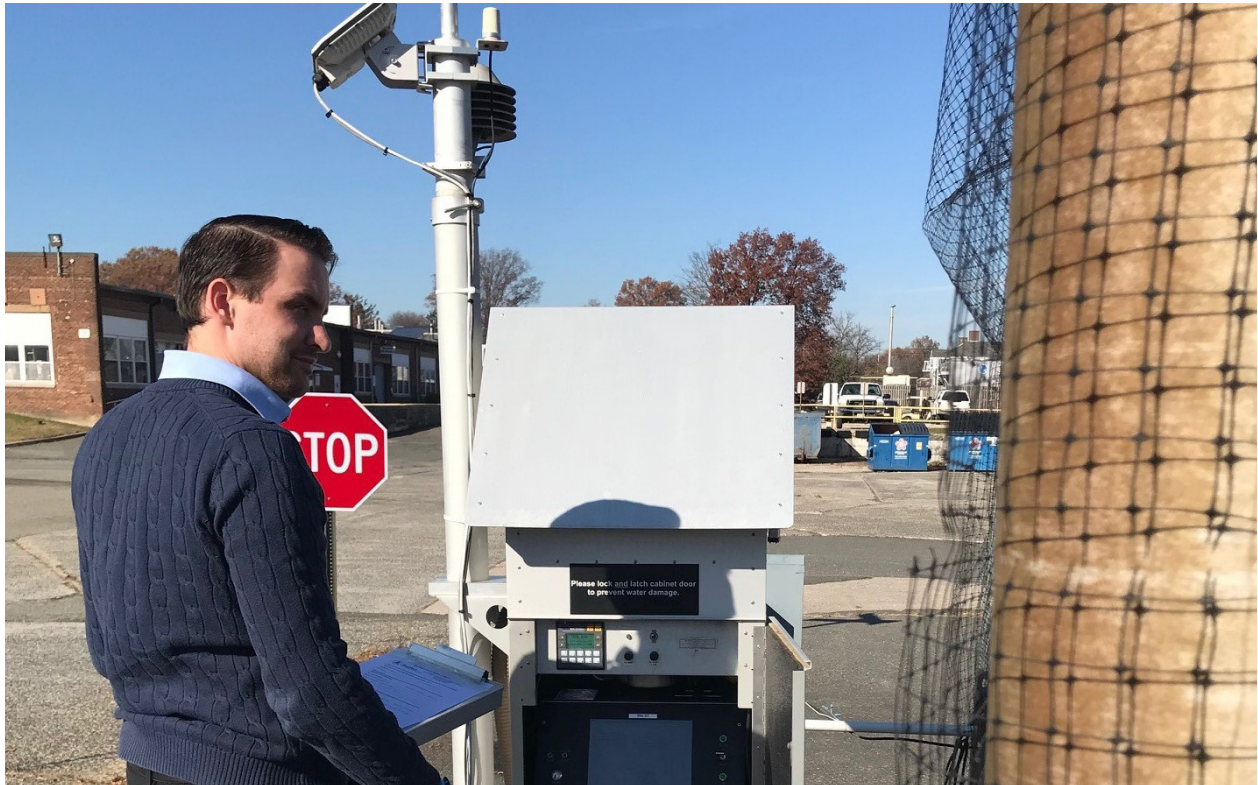
Servicing the RadNet monitor in Edison, New Jersey.
