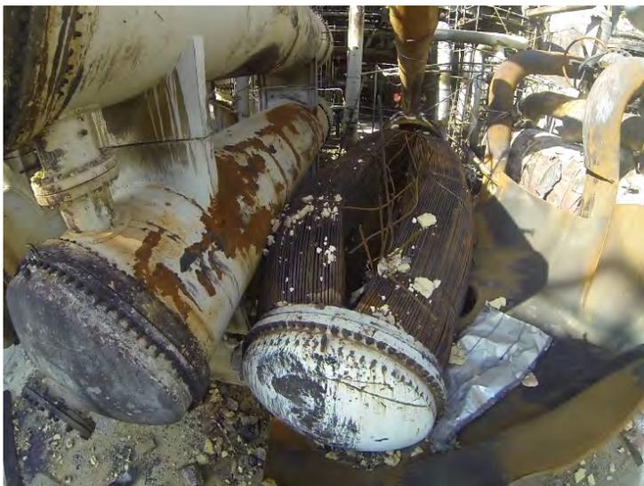
Figure 3 Reboiler, post-accident
