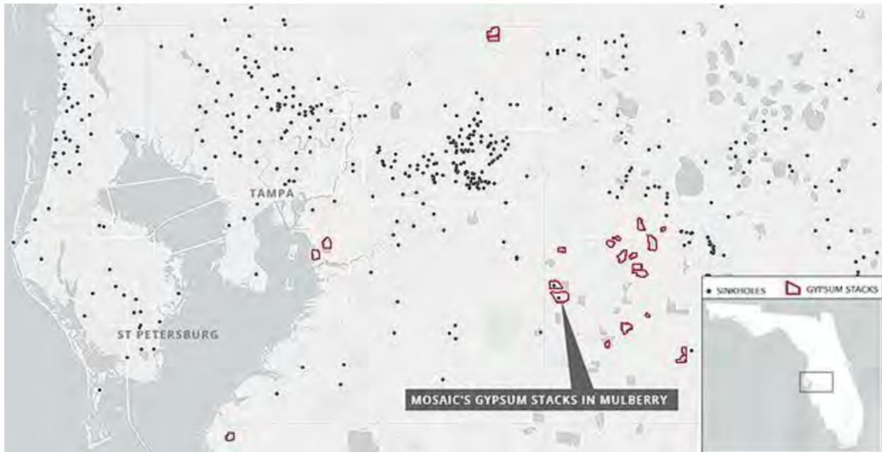
Location of phosphogypsum stacks in West-Central Florida among reported sinkholes from the Florida Geological Survey’s subsidence incident reports database. The area is known as “Sinkhole Alley.” Graphic: Claudine Hellmuth/E&E News (2020).
