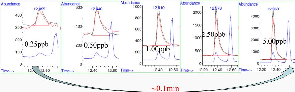
Peak retention time shift and tailing effect:✓ Polar analyte by a nonpolar column
