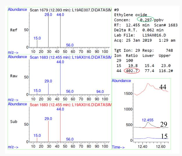
✤Example sample spectra and chromatograms Ion 44 not ideal for quantitation ightarrow Ion 44 – a lump and unresolved peak ► Ion 44 Abundance ratio to ion 29 extremely high  $\sim 4 \mathrm{x} \mathrm{ICAL}$
