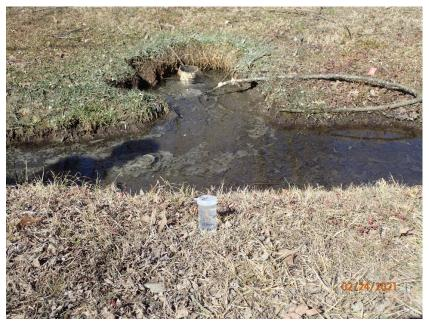
Description: EPA took sample S01 at 11:04 A.M. from the discharge from the cleanout on North 82<sup>nd</sup> Street. Location: North 82<sup>nd</sup> Street SSO.
